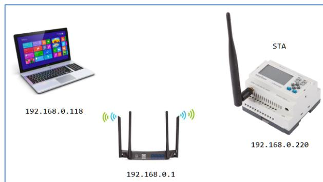
The PLC is used as a Server. The Wi-Fi module works in Server mode.
