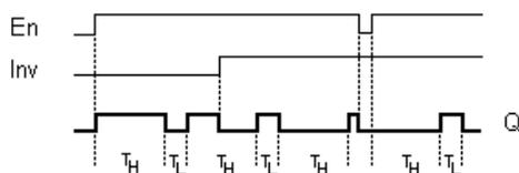
You can set the pulse/pause ratio at the T<sub>H</sub> (Time High) and T<sub>L</sub> (Time Low) parameters.
