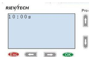
C. Press "OK" for 3 seconds to enter into edit mode.
