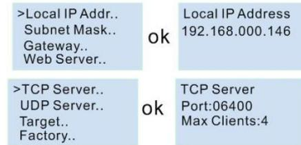
Use these settings in the xLogicsoft Communication Configuration window to enable connection to the CPU from the PC.
